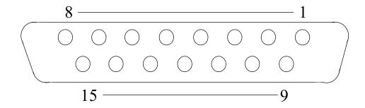
Pin 1 = Mic 1 Gain Pin 9 = +15VDC
