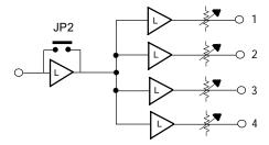
The Model MX401 has one line input and four line outputs. The input gain can be increased by 6dB by removing push-on shunt at JP2. The outputs have adjustable gain.
